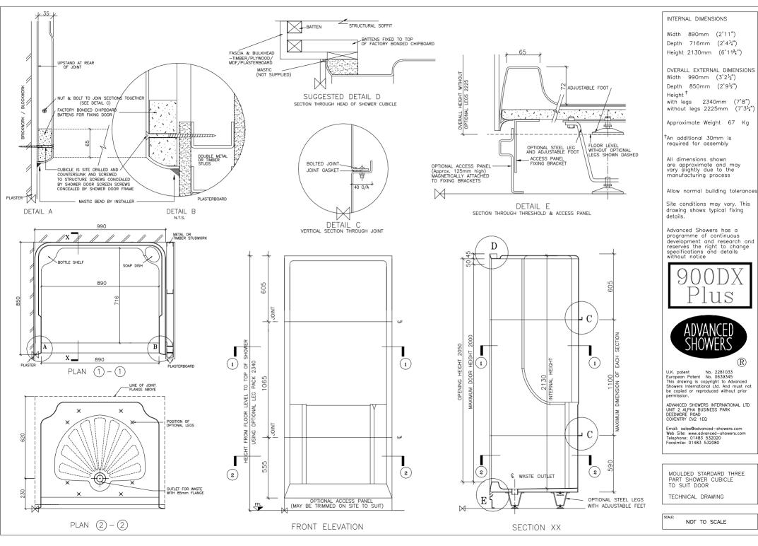
Width 890mm (2'11") Depth 716mm (2'41/4") Height 2130mm (6'11%")
