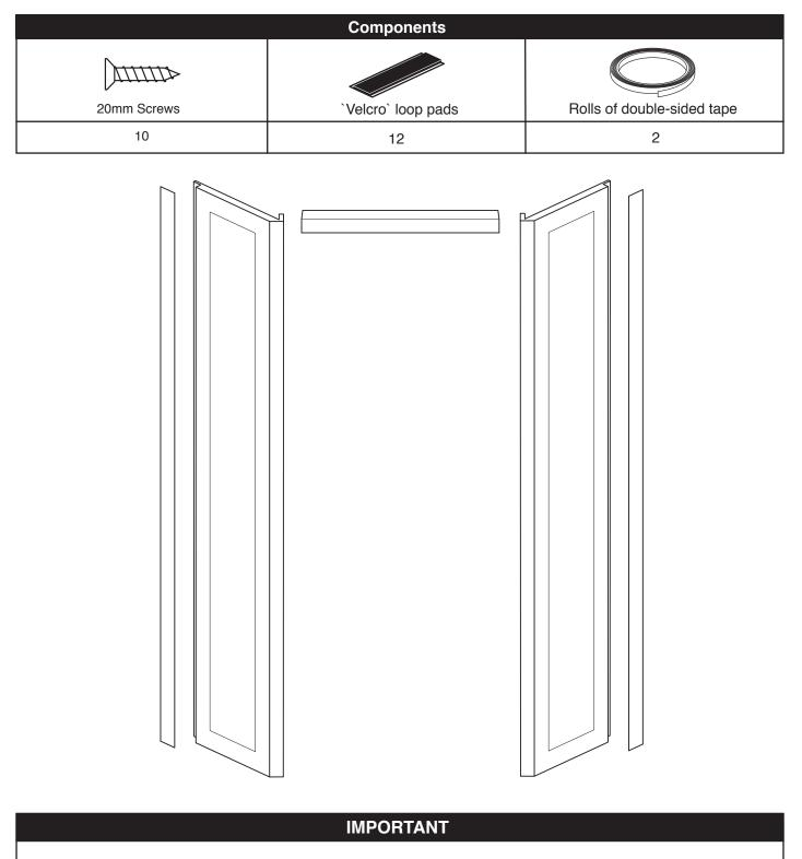
Only for use with the 900SC and 900SD shower cabinets (900SC model shown). Ensure all surfaces to be stuck (self-adhesive 'Velcro' pads, double sided tape or silicone mastic) are thoroughly cleaned first. Fix vertical wall battens (not provided),
